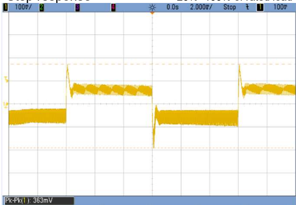
Step response 20%~100% of rated load
