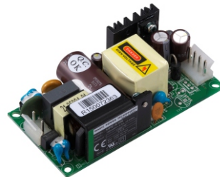
MPE-S13x 130W forced air/100W convection-cooled 12, 24, 48V with optional output 5Vsb Compact size 2" x 4"
